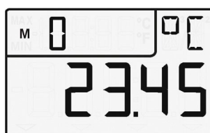
Measured value display, channel M0, temperature
