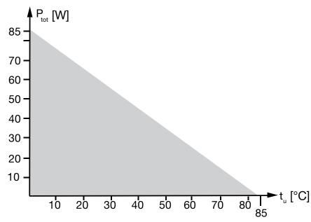
At an ambient temperature of 85 °C, no more than "0 W" is allowed to be input (in theory).
