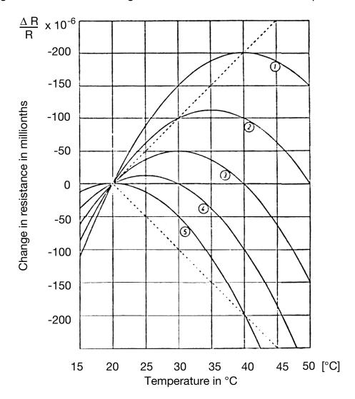
The differences 1 ... 5 in the curves are caused by different production batches for the material (small changes in the alloy composition or its treatment e.g. different rates of cooling).
