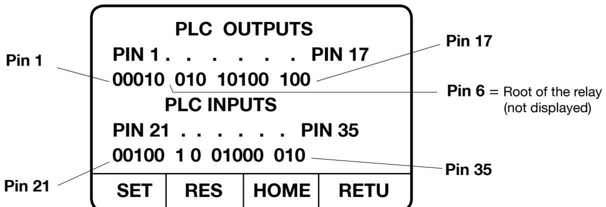
This menu is used to test the PLC interface. The input levels are indicated, and the output levels can be set and reset here.
