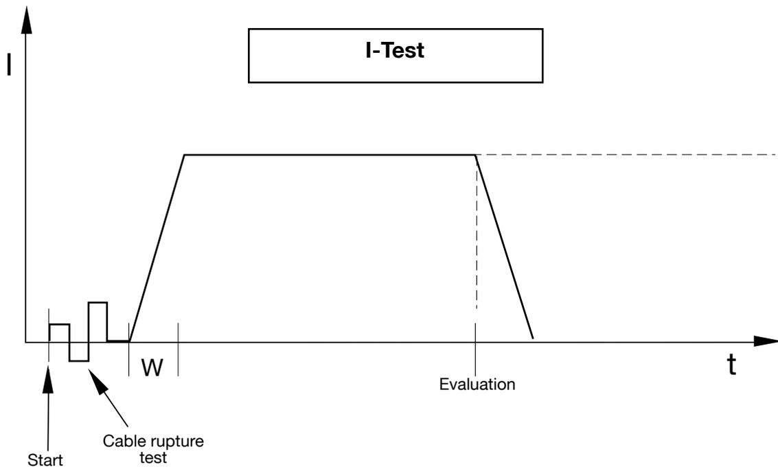
This measurement procedure is only a measurement current monitoring (continuity tester).
