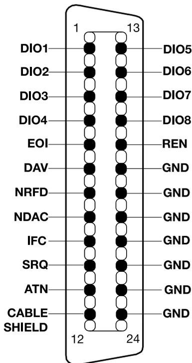
The 24-pole IEEE488 bus plug-connector is standardized and has the displayed pin assignment.
