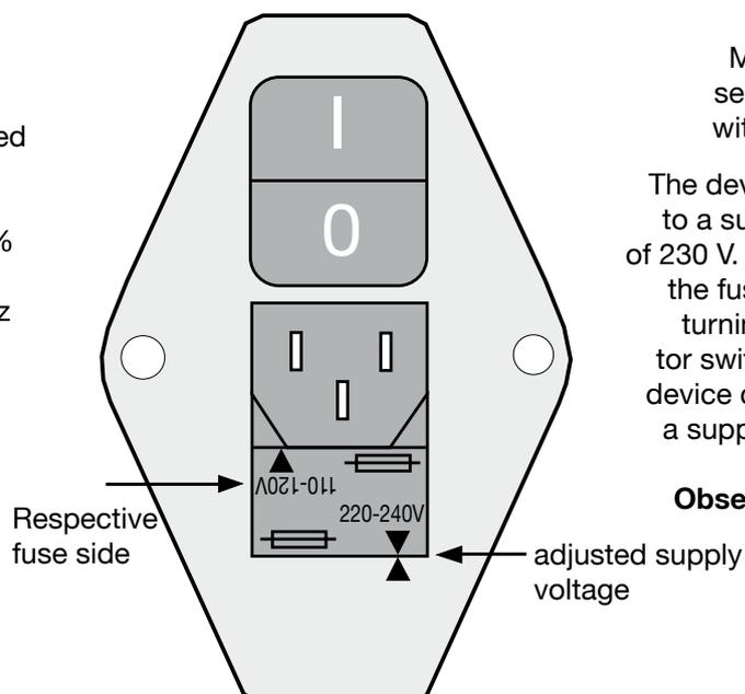
Mains voltage selector switch with fuse catch
