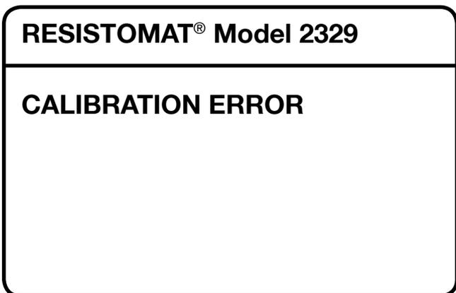
The announcement "Calibration Error" appears on the display when the calibration datas are lost (e.g. when the internal battery is defect).
