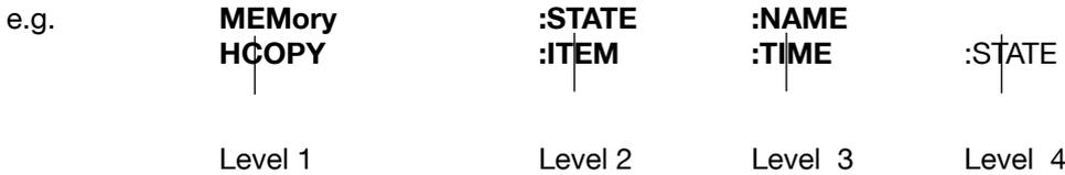
The different command levels are separated by a ":". Some commands have optional headers. For example, the command INITiate:IMMEDIATE has an optional header "IMMEDIATE" on level 2. Optional headers need not be transmitted with their related commands.
