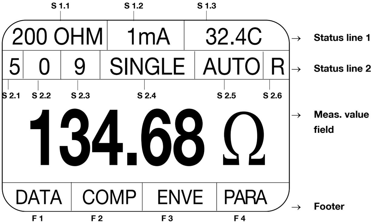
Display with a measurement in progress
