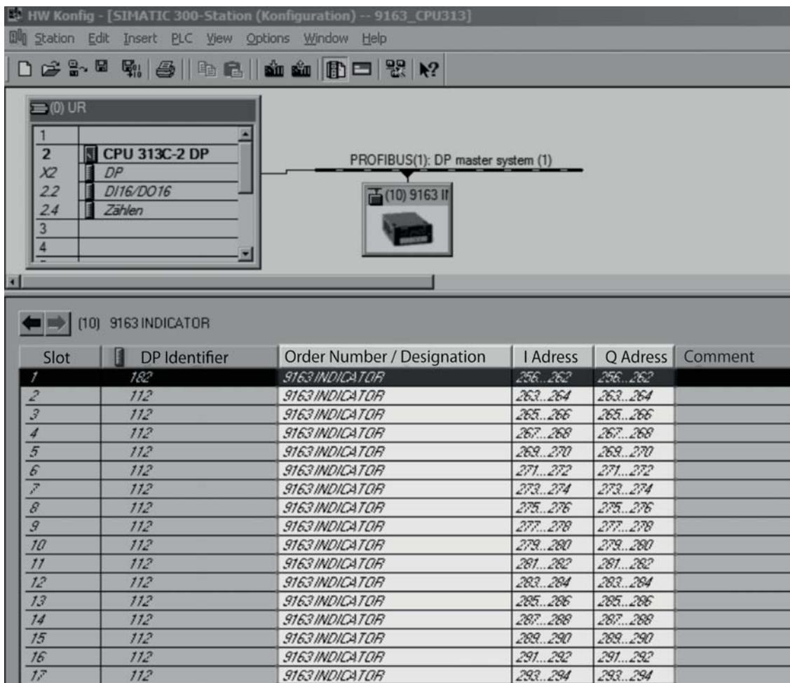
The first 7 bytes, starting at address 256, contain parameter data. These are followed by 32 bytes of process data.
