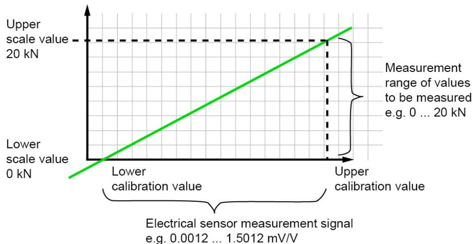
Diagram 27: Scaling of analog sensors
