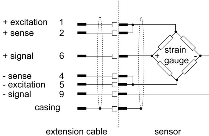
Make the connections between the sense lines and excitation lines as close as possible to the sensor.
