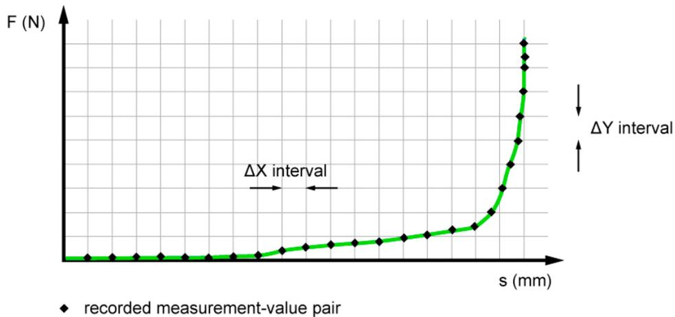
Diagram 4: Sampling methods for the measurement signals
