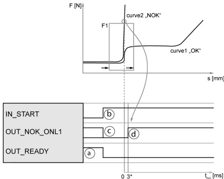
\* The signal sampling method used may increase the typical delay shown here.
