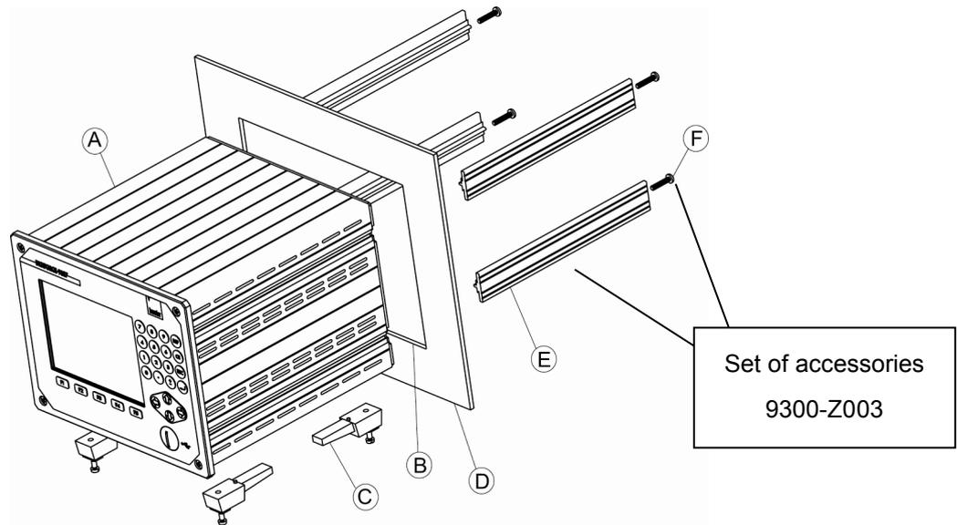
Diagram 20: Instrumen installation
