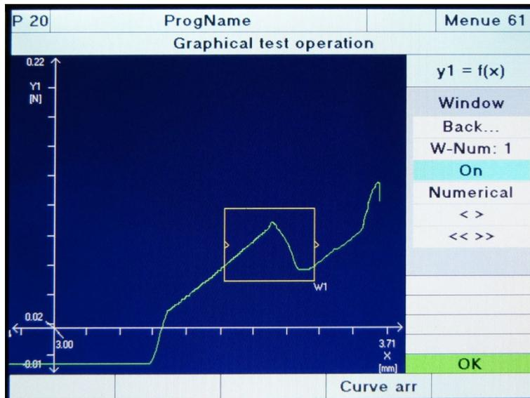
Diagram 49: Graphical test operation – Configuring windows
