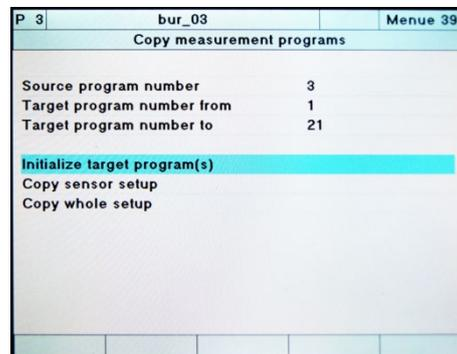
3 Under "Target program number from" or "Target program number to", enter the measurement programs that you want to delete. If you only want to delete one measurement program, enter the same number for "Target program number from" and for "Target program number to".
