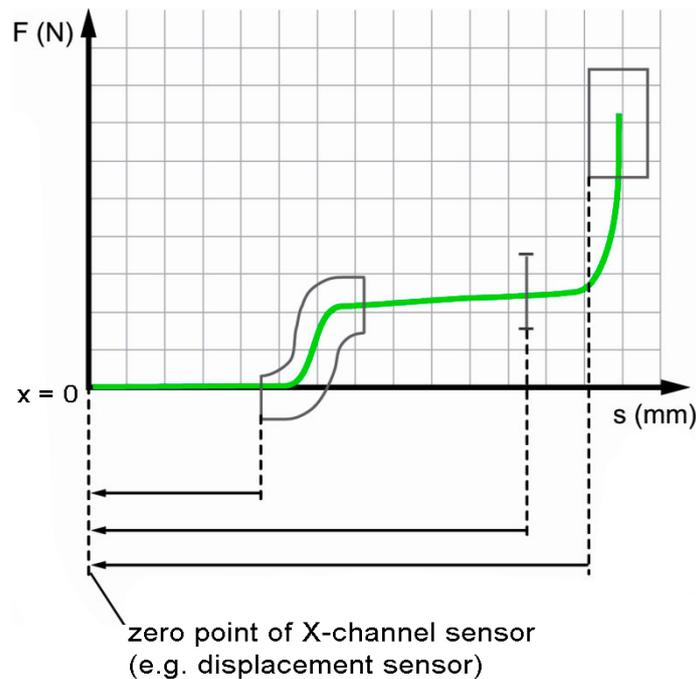
Diagram 6: Measurement curve with ABSOLUTE reference (example)
