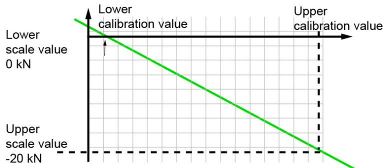
Diagram 28: Inverting measurement signals
