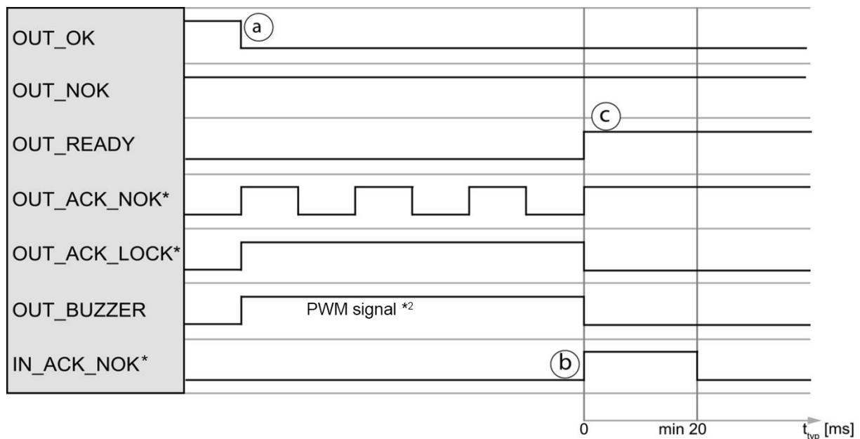
\* You can define a user-configurable PLC output for the signals "OUT\_ACK\_NOK" and "OUT\_ACK\_LOCK".
