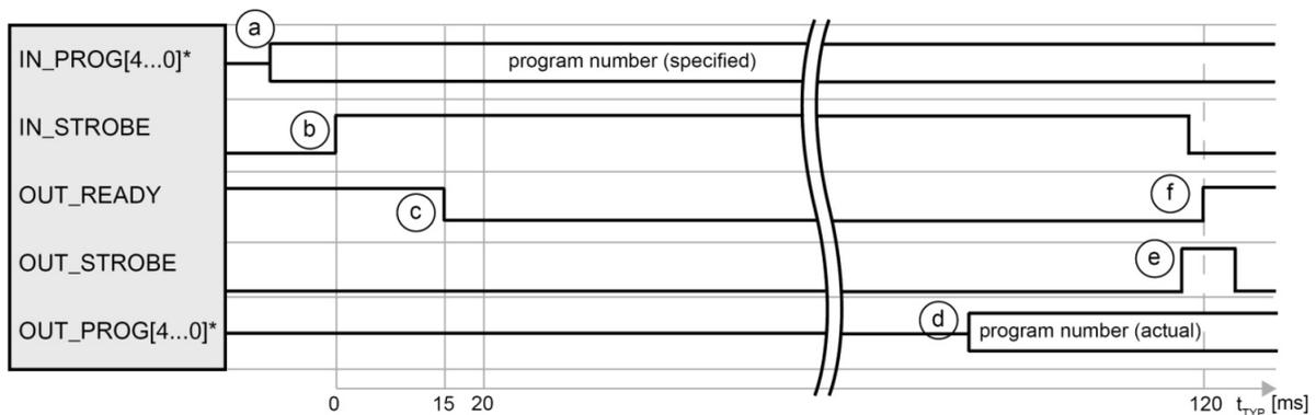
\* IN\_PROG[6..0] and OUT\_PROG[6..0] for 128 measurement programs. You can define a user-configurable PLC output for the signal "OUT\_PROG[6..0]".
