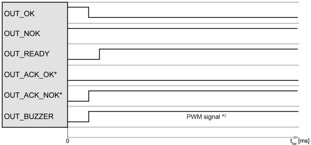
\* You can define a user-configurable PLC output for the signals "OUT\_ACK\_NOK" and "OUT\_ACK\_LOCK".
