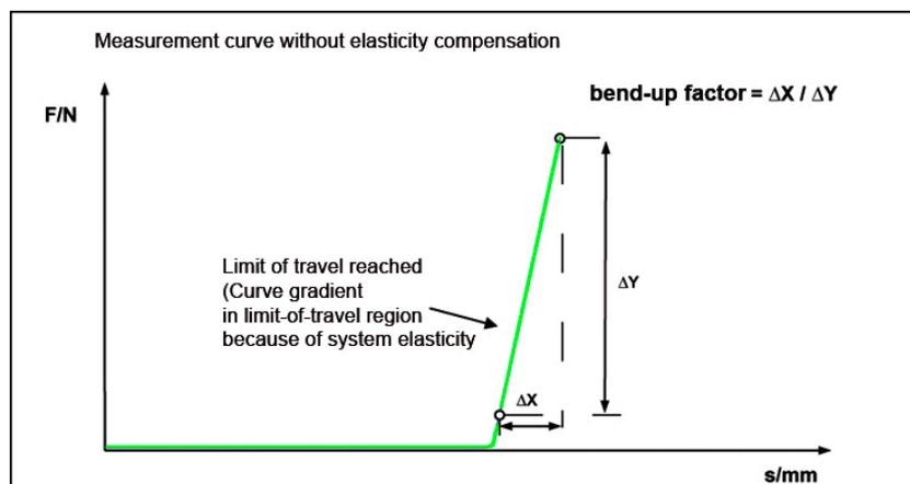
Diagram 33: Finding the bend-up factor from a limit-of-travel measurement without workpiece
