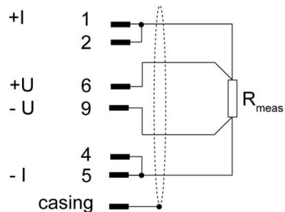
Note: In the 200 mΩ range, use two dual conductors of large cross-section to connect the "+I" and "-I" excitation to  $R_{\text{meas}}$ .
