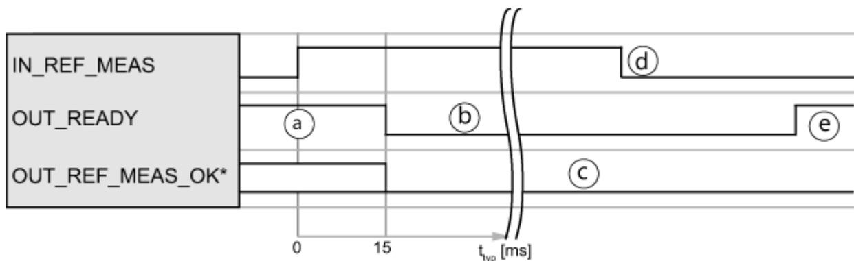
\* You can define a user-configurable PLC output for the signal "OUT\_REF\_MEAS\_OK".
