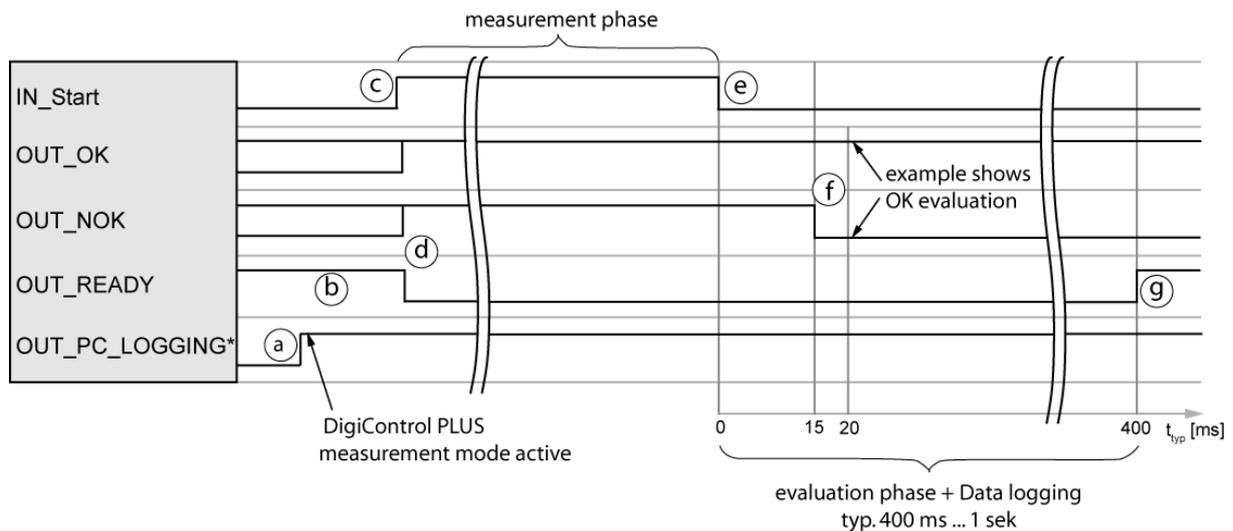
\* You can define a user-configurable PLC output for the signal "OUT\_PC\_LOGGING".
