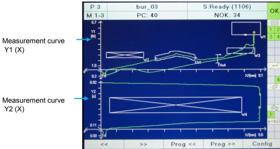
Diagram 60: Measurement curve graphs  $Y_1$  and  $Y_2$  (M1-3)
