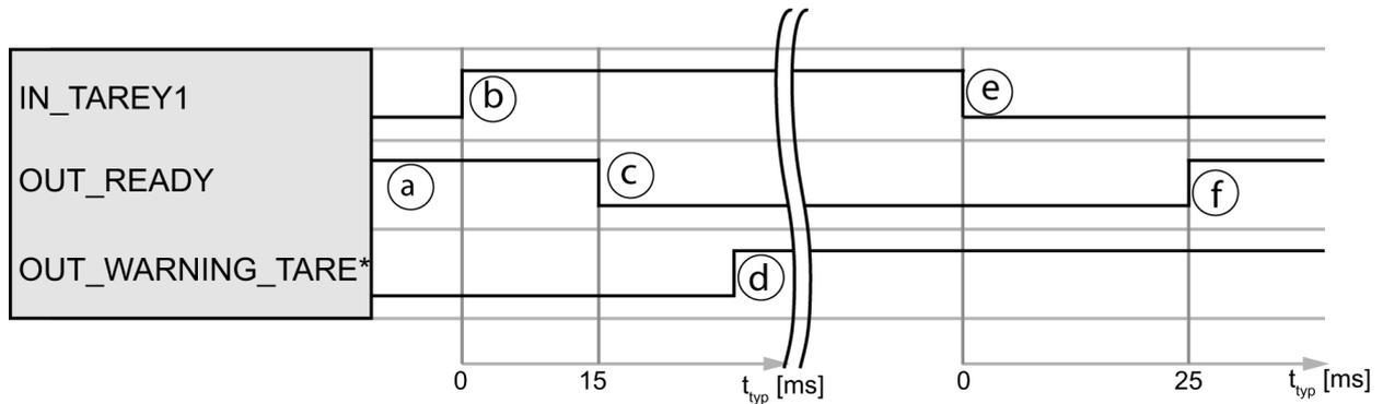
\* You can define a user-configurable PLC output for the signal "OUT\_WARNING\_TARE".
