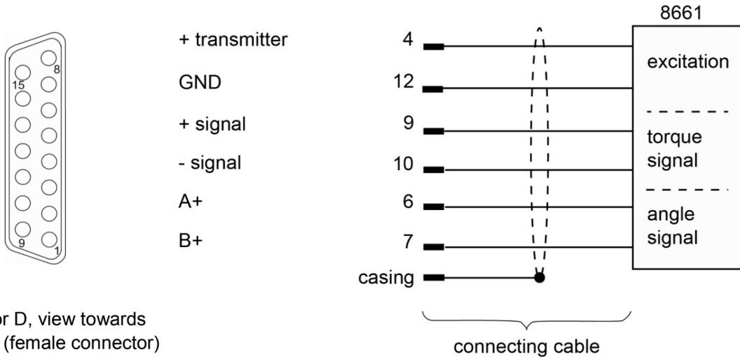
We recommend using the burster connecting cable, model 99163-540A-0150030 (length 3 m).
