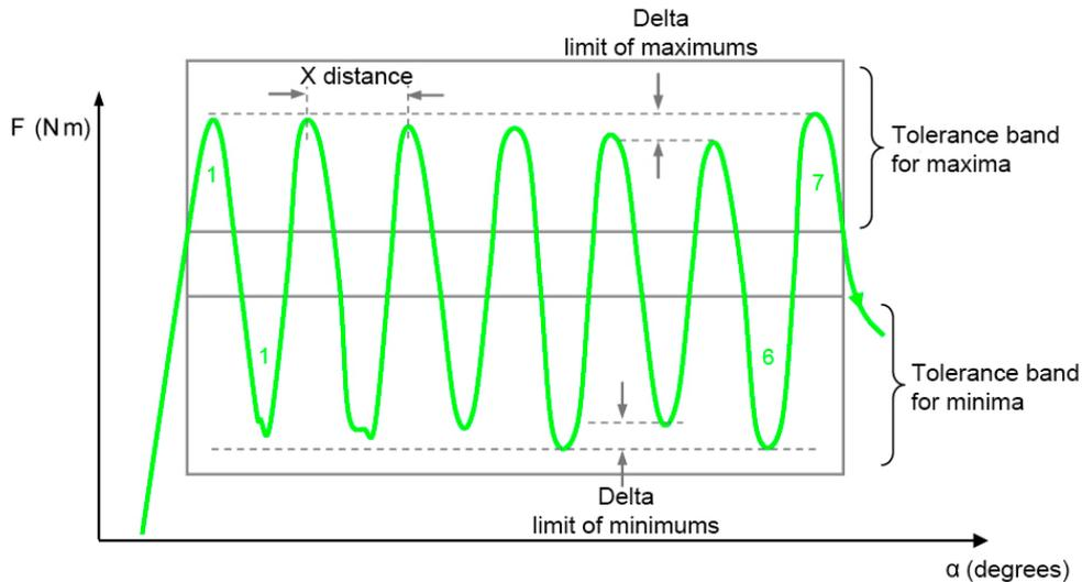
Diagram 44: Rotary-switch testing
