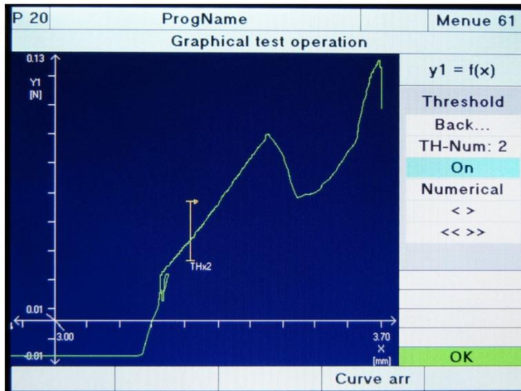
Diagram 51: Graphical test operation – Configuring thresholds
