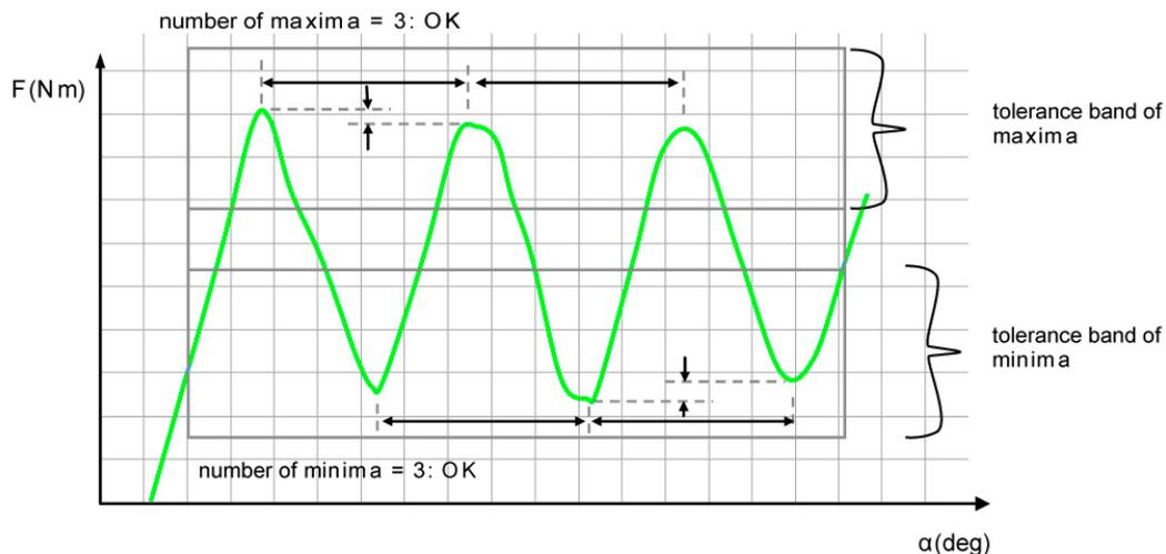
Diagram 13: Rotary switch evaluation
