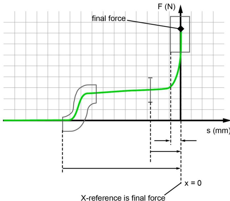
Diagram 8: Measurement curve with FINAL FORCE reference (example)
