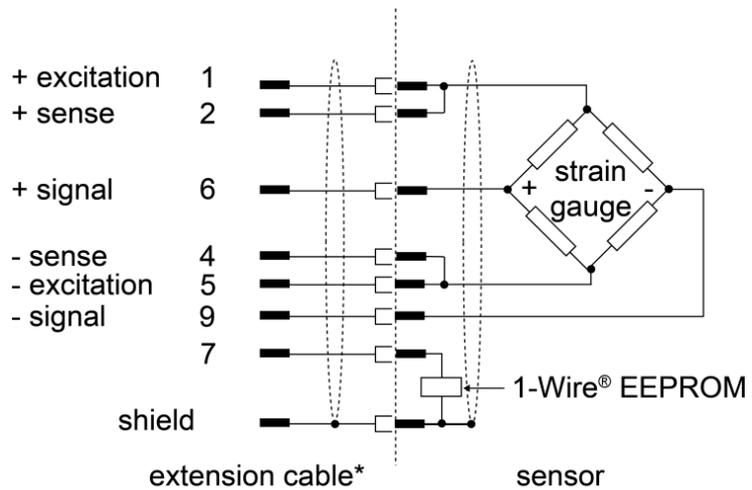
\*Please ensure, that the 1-Wire® signal has to be connected when using an extension cable.
