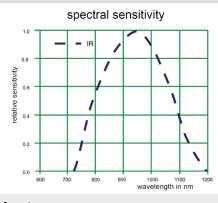
• This measures the solar spectrum in the short-wave IR range (excluding the visible range).
