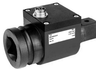
Rotating torque sensor (slip ring) e.g. with square terminal 1 to 5000 Nm
