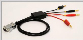
Option 143-60 Cable adapter is designed for simulation of RTD temperature sensors. The adapter is connected to the front panel AUX connector. Platinum and nickel sensors temperature dependency is predefined in the calibrator.
