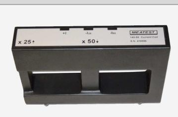
Option 140-50 Current coil with multiplying coefficient x25 and x50 is a useful tool for calibration of clamp ammeters up to 1000 A at 50/60 Hz signal frequency.
