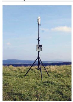
Universal mobile weather station for measuring a wide range of meteorological data, e.g. wind direction, wind velocity, temperature, atmospheric humidity, atmospheric pressure, rainfall quantity and intensity, and global radiation Quick and easy to install, robust design, compatible with various ALMEMO® V7 data loggers.
