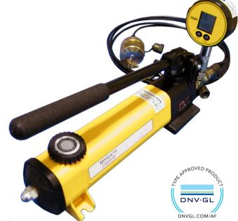
The **PCA205M** - digital pressure calibrator is a microprocessorcontrolled, accurate and versatile digital pressure measuring and calibration instrument with integrated fast peak-, max.- and min.- function. Hydraulic test pressure is generated by the integrated hydraulic pump while read out is done on the digital indicator.
