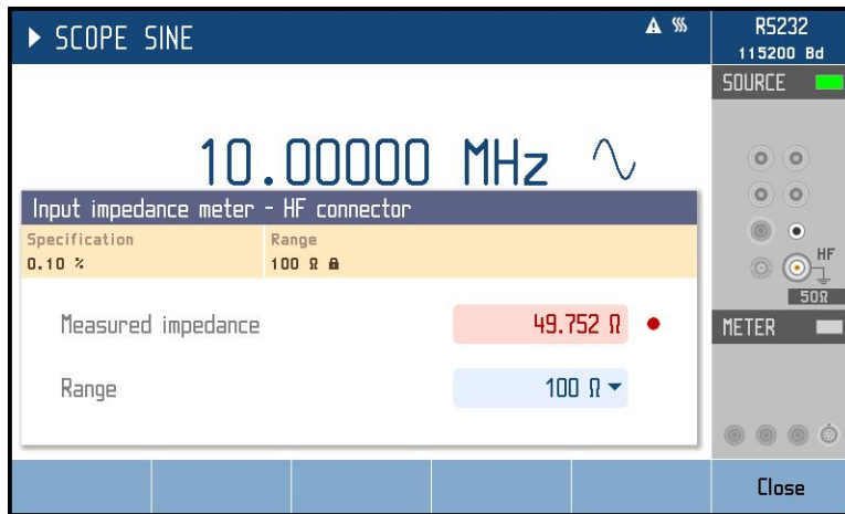
Figure 37 SCO option input impedance measurement
